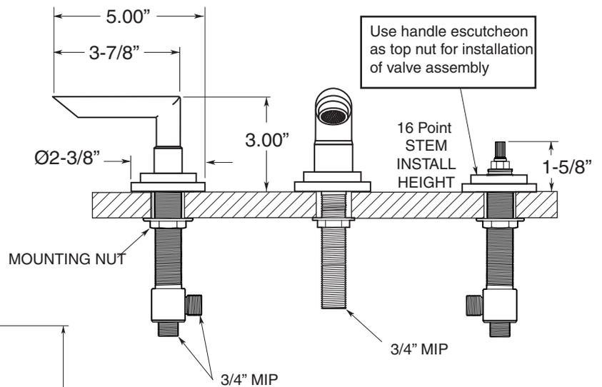
NOTE: Spout and valves install through 1-1/4" diameter holes. Plumber to provide 3/4" supply lines to valves
