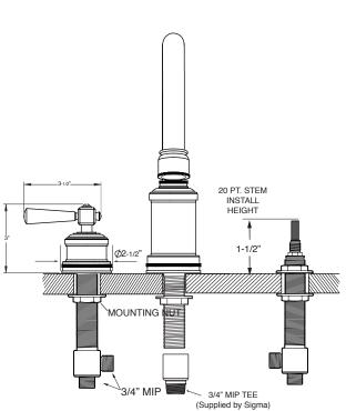
NOTE: Spout and valves install through 1-1/4" diameter holes.
