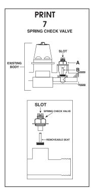
To remove cartridge from body: Rotate cartridge counter clockwise only. To re-set: (Re-seal - Push straight into body and secure with holding nut)
