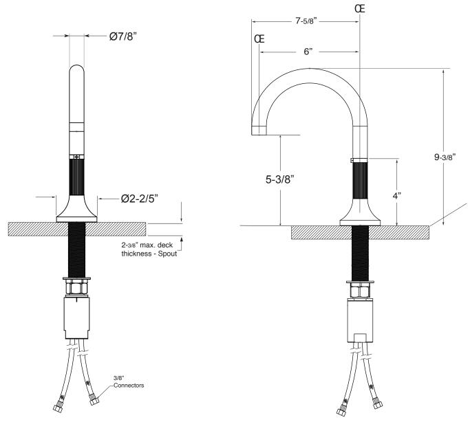
**NOTE**: Spouts install through 1-1/4" Diameter Holes.
