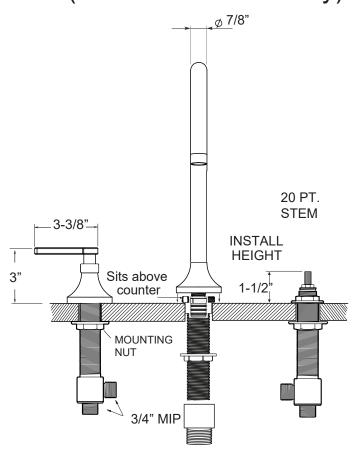
Spout and valves install through 1-1/4" diameter holes. Diverter valve installs through 1-1/2" diameter holes. Plumber to provide 3/4" supply lines to valves
