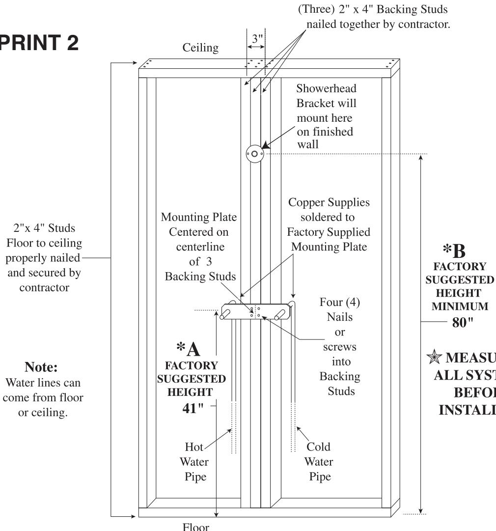
\* Note: These are factory suggestions only - The 80" Height at \*B will allow a 6'5" tall person to walk underneath without bending.
