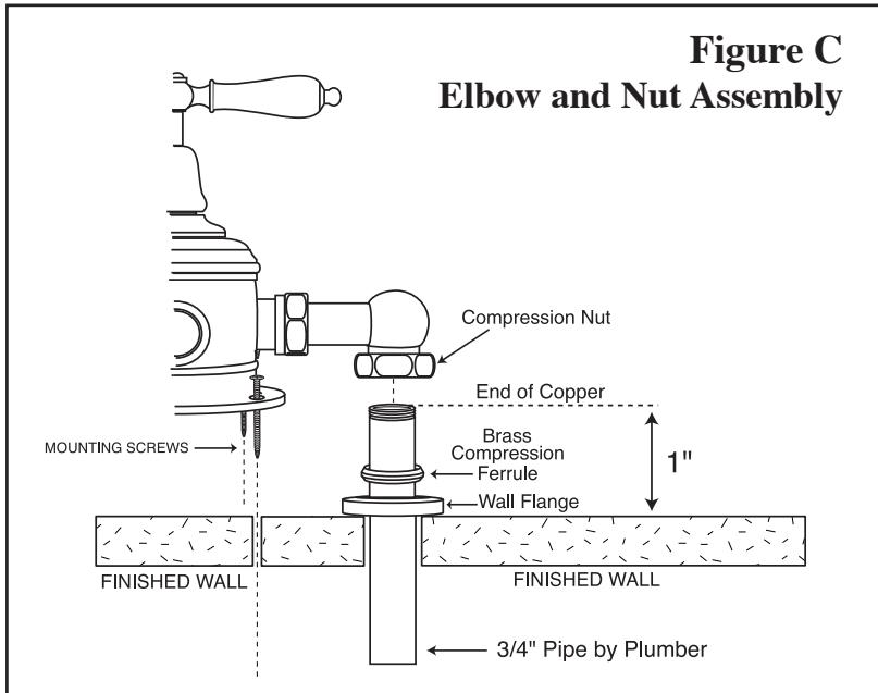
**"Please Note":** The entire valve body must be installed over the copper pipes - **at one time** - do not separate the components.
