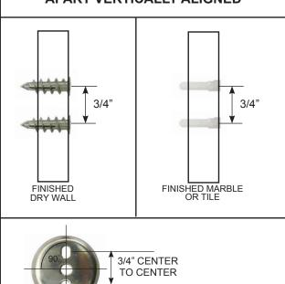
NOTCH IS ALWAYS ON BOTTOM TO HIDE THE SET SCREW HOLE.
