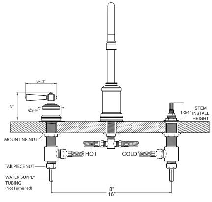
NOTE: Spout and valves install through 1-1/4" diameter holes
