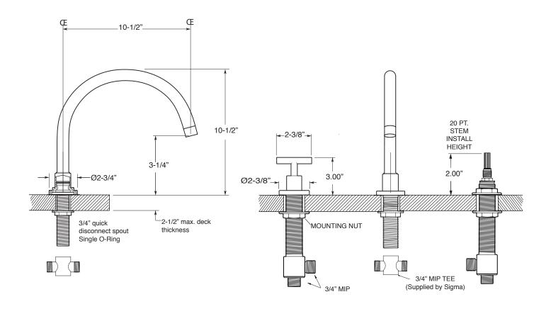
NOTE: Spout and valves install through 1-1/4" diameter holes.
